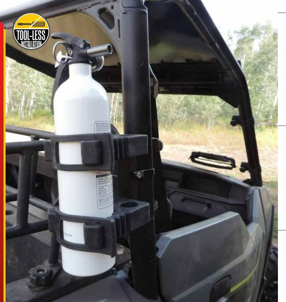
The Hornet Fire Extinguisher UTV Roll Bar mount comes equipped with two heavy rubber grips attached to two large roll bar clamps, making it a simple task to install a fire extinguisher on your UTV.
