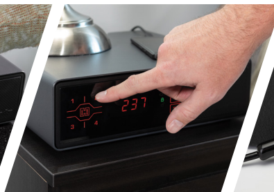
Alternate entry method includes programmable keypad.
