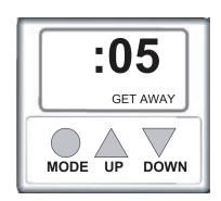
**TEST FEEDER:** PRESS AND HOLD the SET button while the RUN-TIME SECONDS are displayed. Release the button and get away from the feeder when the message "TESTING GET AWAY" appears on the display.
