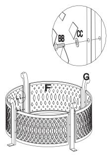
**Step 2:** Attach the Panel (F) with Leg (G) with bolt (BB) and washer (CC). Hand tighten only.
