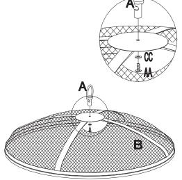
**Step 1:** Attach handle (A) to Mesh (B). Tighten with bolt (AA) and washer (CC).
