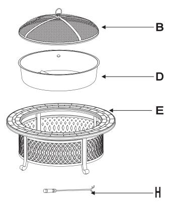
**Step 5:** Turn over the whole assembled piece. Place Fire bowl (D) and Mesh (B) in order.
