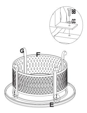
**Step 3:** Attach the Leg (G) with Table top (E) using Bolt (BB) and Washer (CC). Tighten the bolts with wrench.
