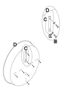
**Step 4:** Put the Grate (C) and Fire bowl (D) in place as below, tighten with Bolt (BB) and Washer (CC).
