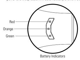
warning: The Hovertrax Prizma/Hovertrax Lux will notify you when the battery charge is dangerously low by beeping. The orange battery indicator light will turn off and the red light will begin to flash. If these warnings occur, immediately slow down and safely step off. Turn the product off. Do not attempt to ride again until the battery is recharged.
