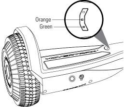
**Note:** To go back to training mode, turn power **OFF**, then press power switch button **ON**. Press power switch button twice **BEFORE** all indicator lights come on.
