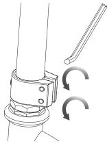
**2** With the front wheel pointed straight ahead and the handlebars square to the front wheel, tighten both bolts on the clamp as shown with a 5 mm Allen wrench. Tighten securely.
