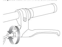
**1** To adjust the brake cable tension, thread the brake lever adjuster in or out 1/4 to 1/2 turn until the desired brake adjustment is attained. Most adjustments are complete at this step. If brake still needs further adjustment, proceed to step 2.
