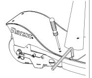
**3** Place the seat post on the deck and secure using the same four (4) screws.
