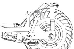
**9** Tighten the cable guide bracket bolt. Tighten the locknuts on the rear axle. Test the brake to verify proper function before riding. Readjust as needed.
