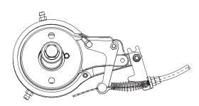
8 Thread the brake cable through the brake adjuster barrel, through the large spring, and into the small hole in the side of the anchor bolt. Position the cable to the original location (as indicated by the slight cable kink) and tighten securely.
