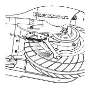
**2** With a 10 mm wrench, loosen the brake cable anchor bolt and disconnect the cable.
