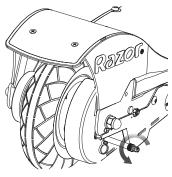
**2** Open the round cover located on the chain guard by sliding the cover downward. Align the opening in the sprocket with the valve stem. Thread the valve extender completely onto the valve stem and attach the pump. Inflate to the PSI indicated on the tire sidewall.
