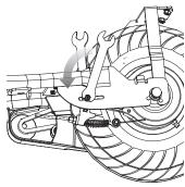
**3** With two (2) 8 mm wrenches, remove the cable guide bracket from the frame and brake plate. Keep the bolt, washer, spacer, and nuts together.
