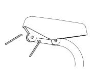
**1** Attach the seat to the seat post with two (2) 4 mm Allen wrenches. See note below.
