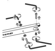
**1** Using two (2) 5 mm Allen wrenches, remove the two (2) coupling bolts from the frame.
