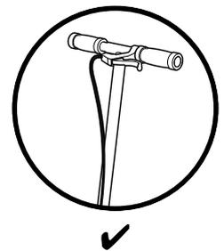
**Note:** The cable assembly from the handlebar must not wrap around the handlebar stem. Sharp bends or twisting of the brake cable can cause the brake to malfunction.
