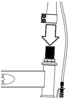
**1** Place the handlebar stem onto the front fork.
