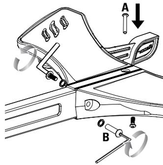
**3** Re-insert coupling bolt (A) first, then re-insert coupling bolt (B). Tighten using two (2) 5 mm Allen wrenches.
