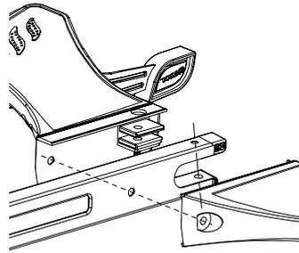
**2** Align the holes on the right and left platforms with the holes on the frame.
