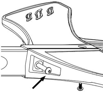
**Note:** If necessary, carefully tap the coupling bolt with a rubber mallet until it is all the way through the other side of the frame.
