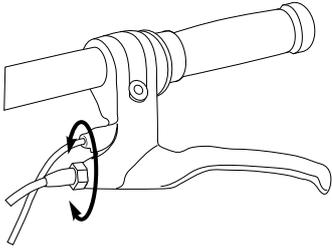
**1** To adjust the brake cable wire, thread the brake lever adjuster in or out 1/4 to 1/2 turn until the desired cable tension is attained.
