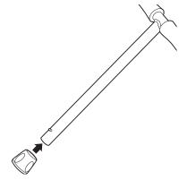
**3** Slide the steering clamp cover onto the T-bar.
