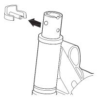
**2** Remove the "E" shaped fixed pin from the front fork assembly.
