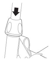
**6** Slide the steering clamp cover down and over the "E" shape fixed pin.
