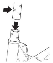
**4** Insert the T-bar into the front fork assembly using your thumb to depress the button on the T-Bar until it "locks" into place.
