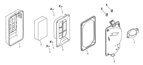
GPA Parts No. LCT Parts No. **DESCRIPTION** Qty GN12000-N-01 1 PGH62600 AIR CLEANER COVER COMP GN12000-N-02 1 PGH62600.2-2 AIR CLEANER ELEMENT. GN12000-N-03 PGS40003 HEX HEAD BOLT M6X12 4 GN12000-N-04 1 AIR CLEANER SEPARATOR PGH62600.2-4 GN12000-N-05 PGH62600.2-5 AIR CLEANER SEAL 1 GN12000-N-06 AIR CLEANER CASE COMP PGH62600.2-1 1 GN12000-N-07 PGH64150 **GASKET** 1 GN12000-N-08 2 PGS20000-M6 FLANGE NUT (M6)
