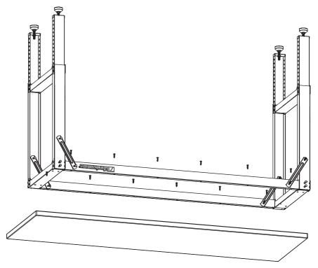
Turn the workbench upright and place in the location it will be used. Check to make sure the workbench is still level. If you need to adjust, use the leveling feet.
