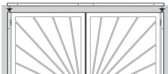
Position the top header jamb (**C**) across the top of the two side jambs. Make certain there is a minimum 1/8" space between the header and the top of the door frame, and that the header is level.
