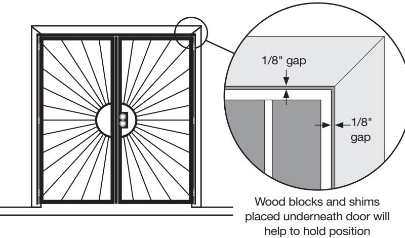
Position the secondary door/hinge-side jamb assembly (**A**) in front of the proper side of the opening. Allow for a 1/8" gap between the edge of door and inside edge of your mounting surface, as well as a 1/8" gap between the top edge of door and bottom edge of your mounting surface. Make certain the assembly is plumb.
