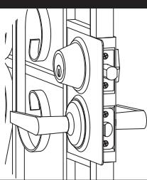
Install your choice of locksets with 2-3/8" backset (sold separately). Fully extend the lock bolts into the "locked" position.
