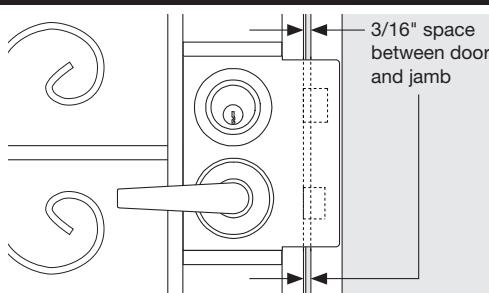
With the lock bolts extended, align the lock bolts with the holes in the lock-side jamb (**B**). Allow approximately 3/16" space between the door and the jamb. Make certain the jamb is plumb, and the top is level to the top of the hinge-side jamb.
