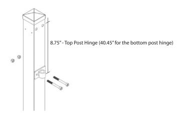
Next, mount gate side of hinge into existing holes in the gate. Mount the bottom post hinge on the post with nuts and bolts included. Do the same for the top hinge. Install gate by hooking the bottom gate side hinge into the bottom post hinge, and the same for the top. Once connected, bolt into place.
