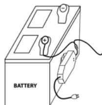
other hot, sharp, moving or pinch parts to avoid damage to the insulation. Secure the AC cord using a cable tie or equivalent. If you have difficulty connecting the output leads, consult your local auto supply store, they may assist you in finding a connecting device for your application.
