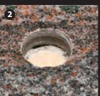
Material: 1/2" granite slab Hole size: 5/8" Power tool: 18v power drill
