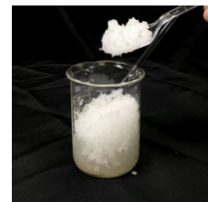
In minutes, slurry turns into a solid for safe transport & disposal.
