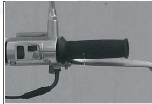
Check whether the acceleration handgrip turns flexibility. If not, it is necessary to clean the accelerator or change the steel cable.
