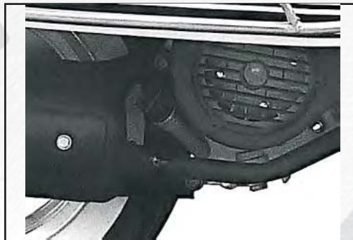
Level the motorcycle and check the oil gauge to see whether the oil level is between the upper and lower markings.
