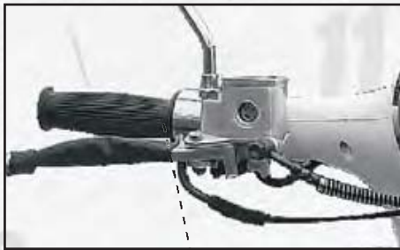
Front braking handgrip: controls the running speed of the front wheel of the motorcycle.
