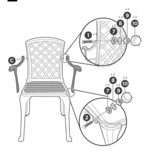
Attach the bottom of the armrest with a part 2 bolt, part 7 washer, part 8 spring washer, part 9 nut, and part 10 nut cap. Repeat to attach the other armrest.
