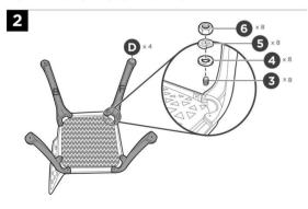
Attach four part D chair legs with eight part 3 fastener, eight part 4 washers, eight part 5 spring washers, and eight part 6 nuts-two washers, spring washers, and nuts perleg.
