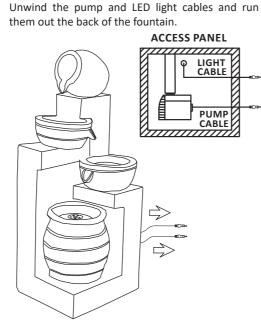
**2.** From the access panel in the back of the fountain, locate the hose and light cables. Attach the pump to
