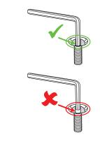
**Tip:** Always fully insert the hex key inside designated notch of the bolt.
