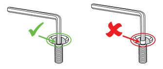
If the hex key is not fully inside the notch, the hex key could slip out, causing damage to the bolt head. Repeated hex key slipping will cause the notch to become rounded, making it difficult or impossible to tighten the bolt with the hex key.
