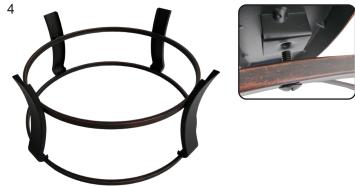
Align Lower Ring (D) with the mounting holes in the middle of the legs; hand-tighten four M6x16mm Bolts (F).
