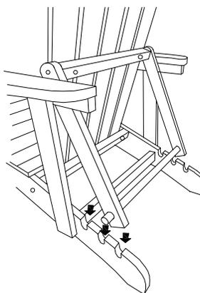
Tighten all nuts and bolts; do not over-tighten as it may damage the finish and crack the wood.
