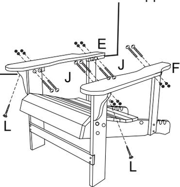
The block on the front of the armrest must be on the outside of the rear arm support.
