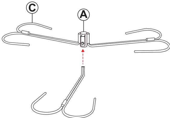
Loosen the bolts on Base Bracket (A).
