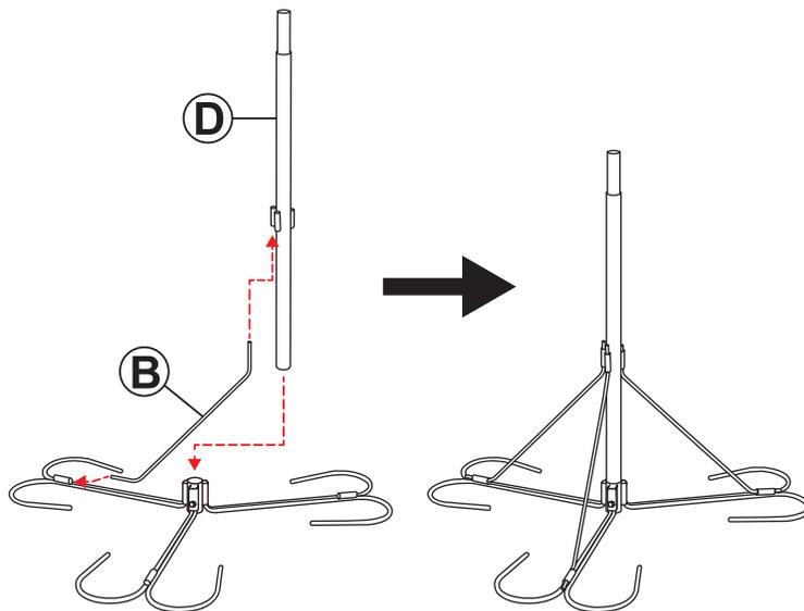
Install Legs (B) into the feet and Bottom Pole (D).
