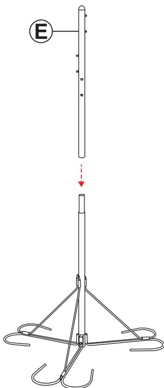
Place Top Pole (E) onto the bottom pole.
