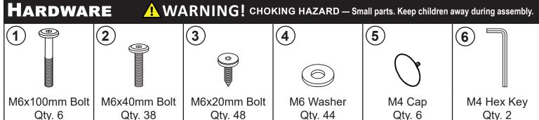
HELPFUL HINT: Do not tighten hardware until all components have been loosely assembled. If the hardware is tightened too soon, mounting holes may not align, and parts may not easily fit together.
