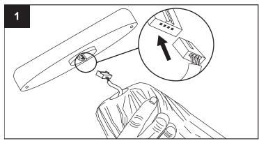
Firmly, but carefully, connect the plug on the solar panel with the socket on the top of the umbrella. Do not pull on wires as doing so may permanently damage the connections.
