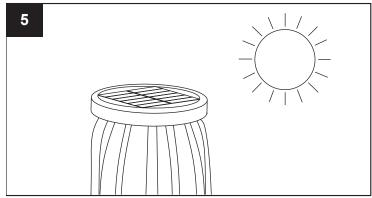
Before the first use, ensure the solar panel receives at least 8 hours of direct sunlight to charge the battery.
