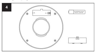
Remove the old battery. Paying attention to the positive and negative terminals, insert the new battery.
