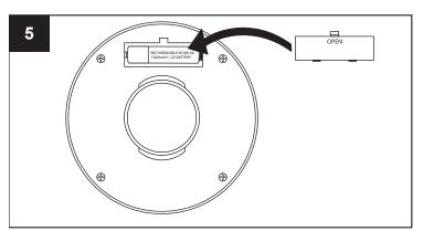
Replace the battery housing cover and reconnect the solar panel to the umbrella.
