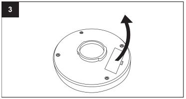
Place the solar panel face-down on a soft, clean surface. Remove the battery housing cover.
