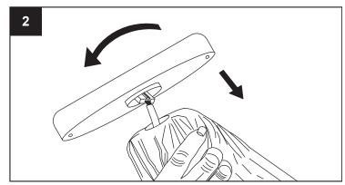
Align the notches on the solar panel with the grooves on the top of the umbrella, hide the plug and wires inside the hollow space. Turn the solar panel clockwise to lock into place; do not over-tighten.
