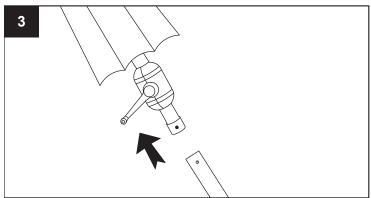
Attach Umbrella (A) to Pole (B) by pushing the button spring clip on the pole and aligning it with the hole on the umbrella. You will hear a 'snap' when the pieces are connected.
