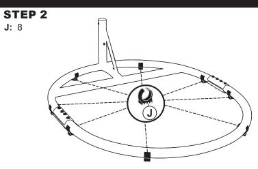
Carefully snap Foot (J) evenly onto the stand base, as shown. **IMPORTANT:** If feet are not evenly distributed the stand could tip over when in use.
