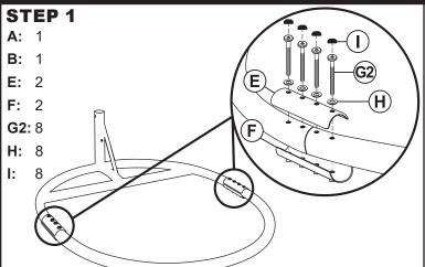
Align Base Back (A), Base Front (B), Top Base Connector (E), and Bottom Base Connector (F) and secure using Washer (H) and M6x50mm Bolts (G2). Place Bolt Caps (I) on the bolt heads.
