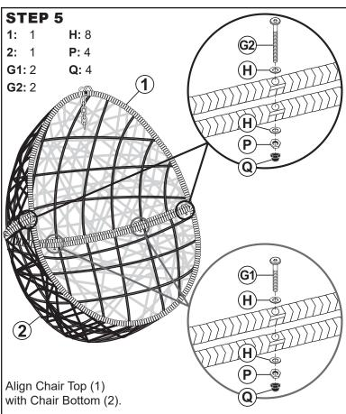
As shown, hand-tighten M6x50mm Bolts (G2), Washers (H) and Lock Nuts (P) to the outside mounting holes. Then, hand-tighten M6x45mm Bolts (G1), Washers (H) and Lock Nuts (P) into the center mounting holes.
