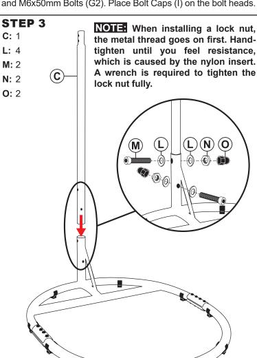
Slide Straight Pole (C) into the back base and align the holes. Secure the pole using M10x60mm Bolts (M), Washers (L), and Lock Nuts (N) as shown. Place Large Hex Nut Caps (O) over the lock nuts.
