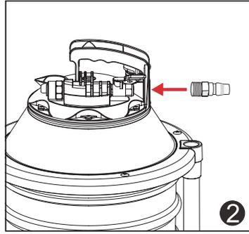
Before use, apply thread tape to the quick coupler before fitting the coupler to the unit.
