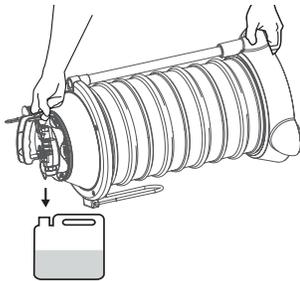
4. After all the oil has been extracted. Turn the lever to the "CLOSE" position and disconnect the air line from the unit. Remove the extracting tube from the dipstick tube (refit the oil dipstick). Remove the main suction tube from the unit. Slowly pour the used oil into a suitable container and dispose of it in an appropriate manner.
