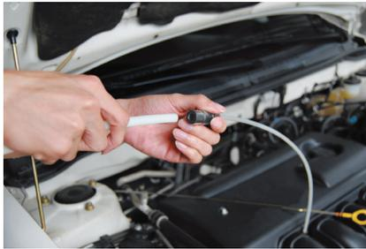
2. Select and insert the appropriate diameter extracting tube into the dipstick till it reaches the bottom of the oil pan, connect the main suction tube to the unit and to the extracting tube.
