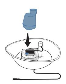
Insert the filter housing into the opening on top of the pump.
