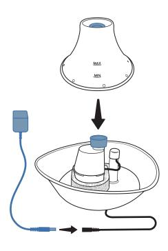
Set the tower down over the filter housing and press down on the silicone gasket to form a seal. Connect the power adaptor.
