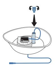
Insert the pump into the foam filter and set both down into the square inside the bowl. Press down so the suction cups attach.
