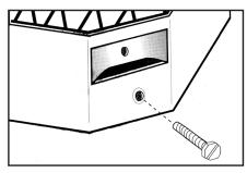
1. Insert one screw into the lower hole located in each mitered corner of the chimney cover band. (Just start the screw into the hole a few turns, until all four screws are started.)
