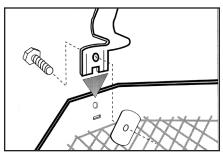
1. Insert the leg inside each corner of the base of the chimney cover until the hole in the leg is aligned with the hole in the base and the rectangular tab on the leg fits into the slot in the base. Insert the mounting bolt (provided with the leg kit) through the hole in the base and the hole in the leg. Hold the self-locking nut against the end of the bolt and twist the bolt until the nut threads on the bolt 2-3 times. **Do not tighten fully at this time.**
