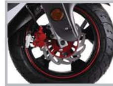
Front Brake Disk With ABS pump
