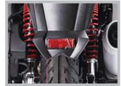
Dual Spring Shocks Robust rear suspension
