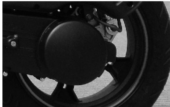
Automatic clutch: automatically controls the separating/meshing of the clutch based on the running speed of the motorcycle.
