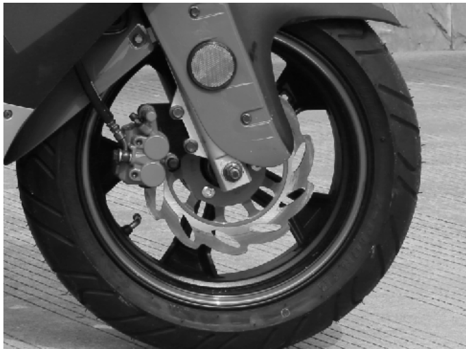
Check the air pressure of the tire and check whether the rim deforms. If any abnormality is found, it should be handled properly.
