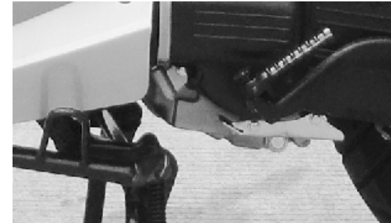
③The Engine Number is printed on the left lower part of the crankcase.
