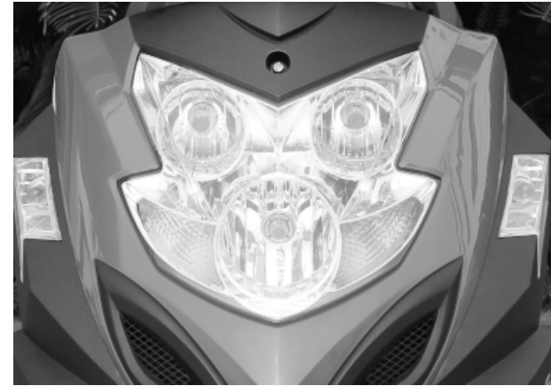
Check whether the head light, turning lights and indicator lamps work properly.
