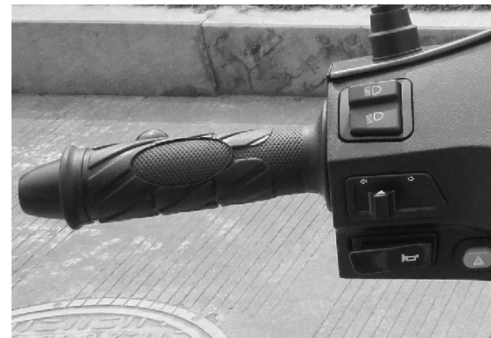
Rear braking handgrip: controls the running speed of the rear wheel of the motorcycle.
