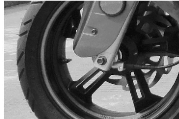
Check the air pressure of the front tire and the wear of the tire casing.
