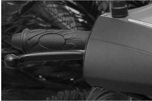
Check whether the free travel of the front braking handgrip meets the standard 10mm-20mm.
