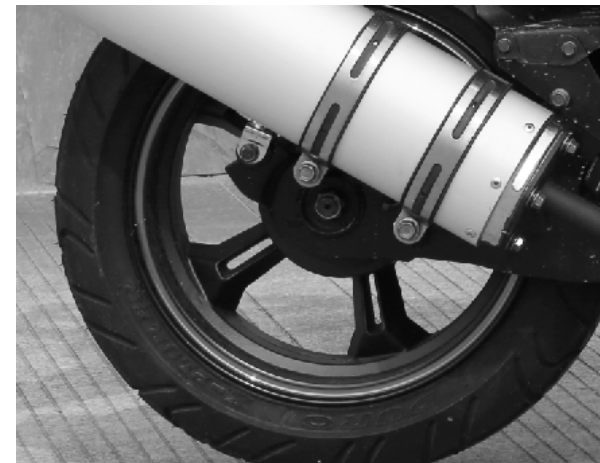
Check the air pressure of the rear tire and the wear of the tire casing.
