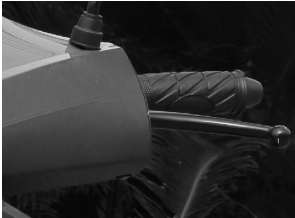
Check whether the free travel of the rear braking handgrip meets the standard 10mm-20mm.
