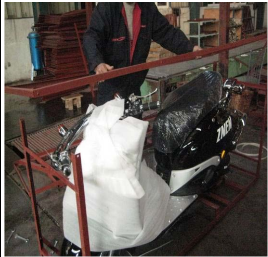
8: Pull upper frame up carefully.
