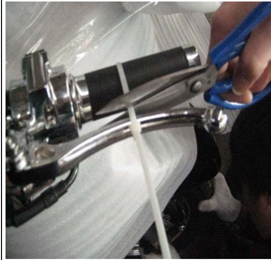
14: Cut ties on brake levers.
