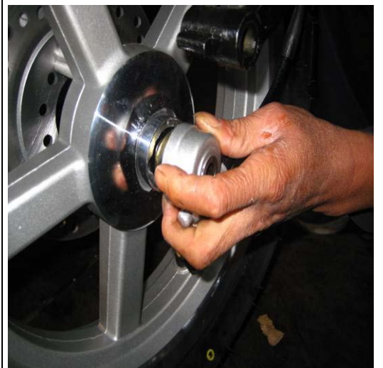
15: Insert spacer, put front wheel & speed sensor in place.
