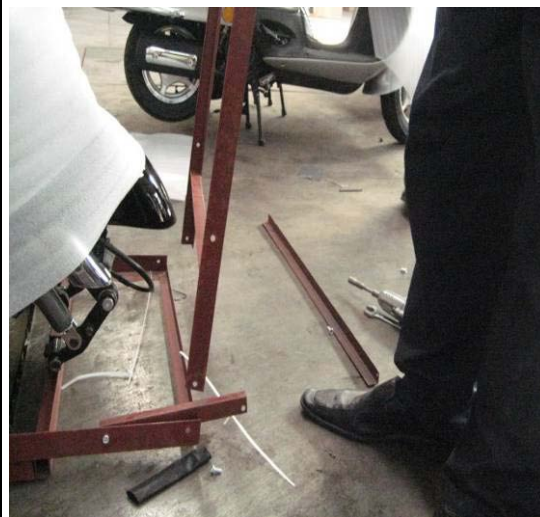
8: Pull upper frame up carefully.
