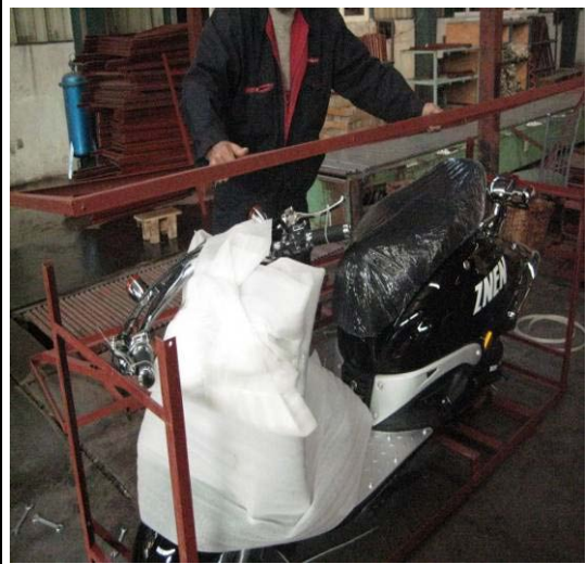
8: Pull upper frame up carefully.
