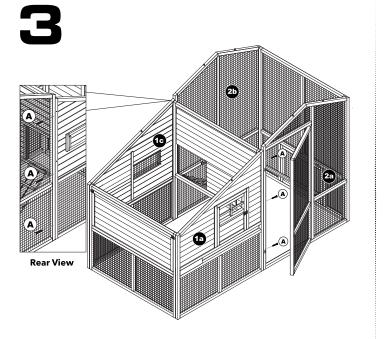
3. Connect Foraging Area Panels **(2a, 2b)** to Roosting Area Panels **(1a,1c)** with Screws **(A)**.
