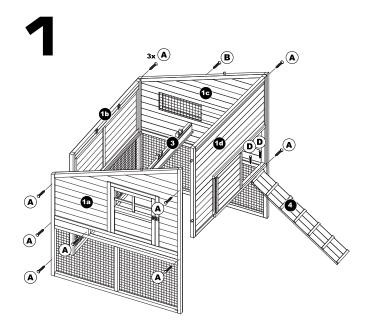
1. Connect Roosting Area Panels **(1a, 1b, 1c, 1d)** with Screws **(A).** Attach Nesting Box Floor Support **(3)** with Screws **(A-On Front, B-On Back).** Attach Ramp **(4)** with Screws **(D).**
