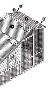
5. Attach Lower Left Roof Panel (7) with Screws (B) and Plastic Washers (E). Attach Upper Left and Right Roof Panels (8 & 9) with Screws (B) and Plastic Washers (E).
