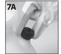
Adjust spray pattern by turning nozzle cap. Do not turn cap more than 2 turns or cap may come off allowing spray material to spray back on you.
