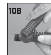
Insert notches from underside of handle into plunger grooves and turn counterclockwise.
