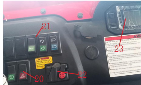
20. Hazard warning light switch 21. Switches 22. 2WD-4WD switch 23. Indicators & Display
