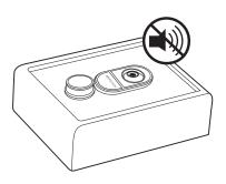
To initiate silent entry mode, hold a programmed finger on the scanner for 5 seconds beyond your fingerprint being accepted. The green indicator ring will turn off and back on, but will not beep, indicating you are now in silent entry mode.
