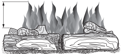
Figure 22 - Incorrect Burner Flame Pattern
