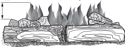
Figure 21 - Correct Burner Flame Pattern
