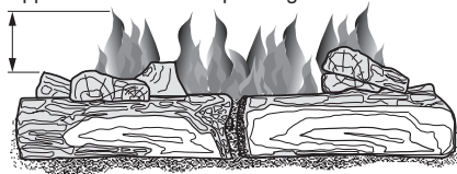
Figure 24 - Correct Burner Flame Pattern
