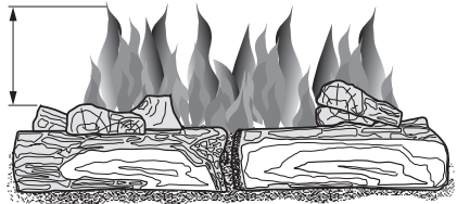
Figure 25 - Incorrect Burner Flame Pattern
