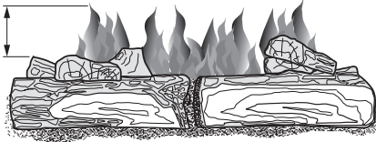
Figure 24 - Correct Burner Flame Pattern
