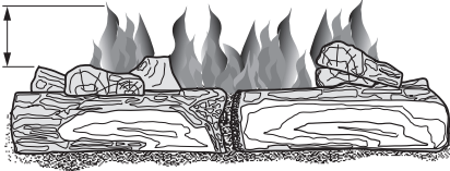
Figure 31 - Correct Burner Flame Pattern
