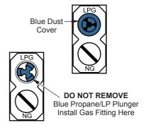
Apply thread sealant to the threads on the connection fitting. While pushing in, rotate the fitting clockwise until the threads engage the regulator. After the fitting has been hand tightened into the regulator use a wrench to complete tightening of the fitting. Install additional fitting to connect to the house supply.
