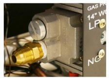
DO NOT use an off the shelf 3/8" NPT pipe plug. This will damage the plungers located inside the regulator.
