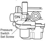
Figure 28 - Gas Regulator Pressure Switch
