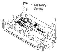
Figure 10 - Attaching Heater Base to Fireplace Floor
