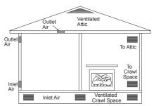
Figure 3 - Ventilation Air from Outdoors
