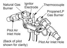
Figure 27 - Pilot Inlet Air Hole
