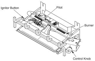
Figure 1 - Vent-Free Log Chassis
