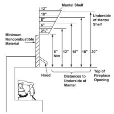
Figure 7 - Minimum Mantel Clearances When Using Hood
