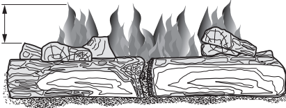
Figure 31 - Correct Burner Flame Pattern
