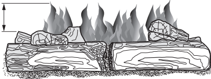
Figure 31 - Correct Burner Flame Pattern
