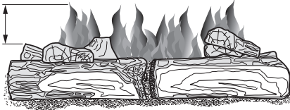
Figure 23 - Correct Burner Flame Pattern
