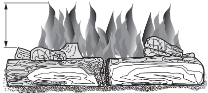
Figure 24 - Incorrect Burner Flame Pattern
