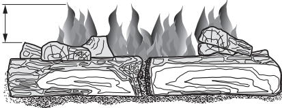
Figure 30 - Correct Burner Flame Pattern
